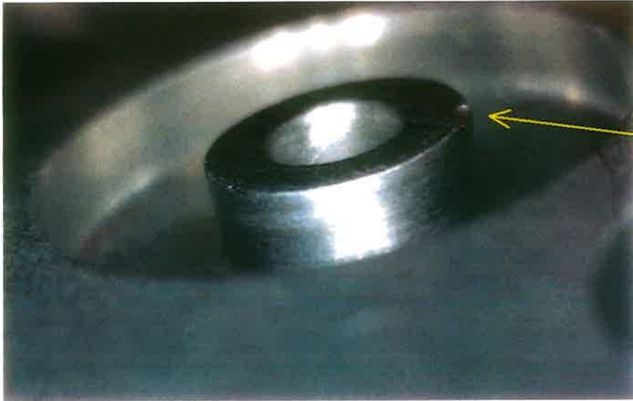
Figure 12 – Ding on Port
