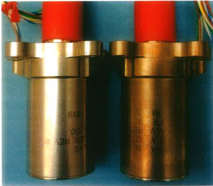
Figure 16 – “Inconsistent” Plating Appearance
