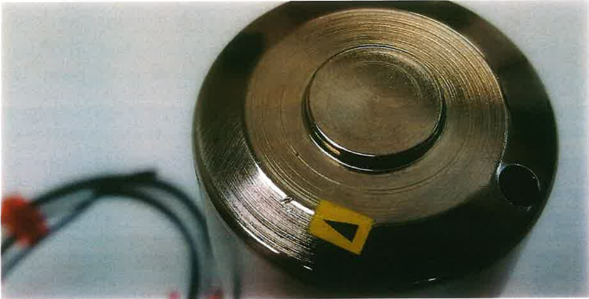
Figure 10 – Ding on Housing
