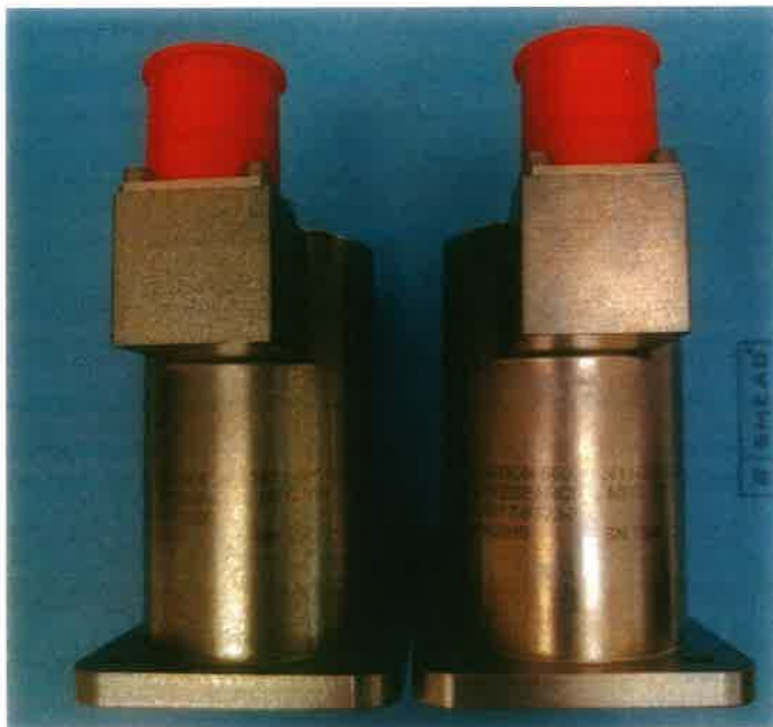
Figure 15 – “Inconsistent” Plating Appearance
