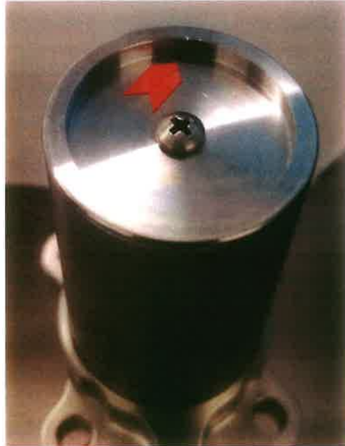
Figure 7 – Dings on Non-Functional Surface
