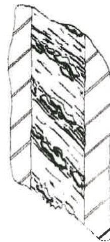
Potentially loose friction welded particles
