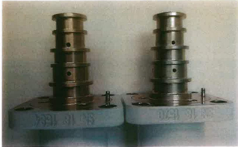
Figure 8 – “Inconsistent” Anodize Appearance
